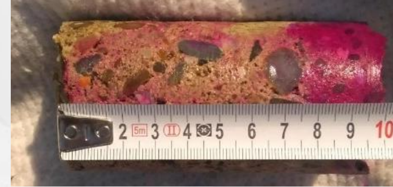
Figure 2. The carbonation depth of concrete at the places where the render was missing – sample selected from the measurements performed in 2018 (Bridge in Sládkovičovo).
