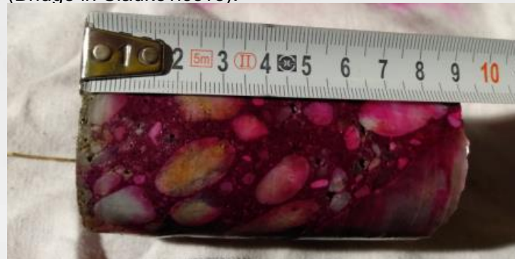
Figure 3. The carbonation depth of concrete at the places with a thin layer of PRC at the surface – sample selected from measurements performed in 2019 (Bridge in Rimavská Sobota).
