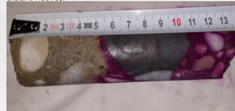
Figure 4. The carbonation depth of concrete at the places where this render was missing – sample selected from measurements performed in 2019 (Bridge in Rimavská Sobota).
