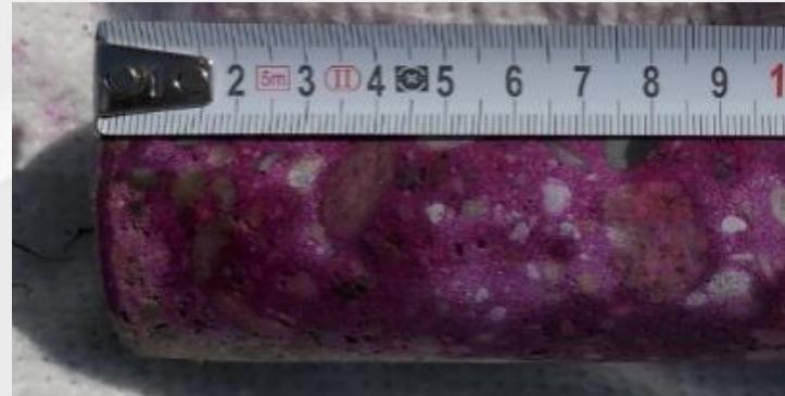
Figure 1. The carbonation depth of concrete at the places with a thin layer of PRC at the surface – sample selected from the measurements performed in 2018 (Bridge in Sládkovičovo).
