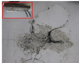
Photo :Serial Number 12-1 (four anchors) at pry-out failure
